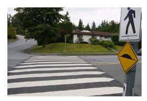
Raised Crosswalk: Another iteration of the crosswalk, the raised crosswalk can be erected on its own or as part of an entire raised intersection. Raised intersections are flush with the sidewalk and ensure that drivers traverse the crossing slowly. Crosswalks do not need to be marked unless they are not at grade with the sidewalk. ADA-compliant ramps and detector strips are always required.
